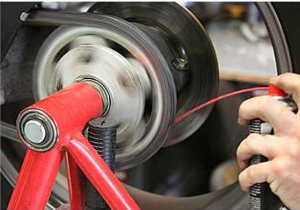
Whether or not your chain needs adjusting, you'll want to keep it clean and well-lubricated. Most modern chains are o-ring types which use rubber components, and are sensitive to certain solvents. Make sure you use an o-ring approved cleaning agent when you spray the chain and sprockets or use a soft brush to apply the cleaner.
