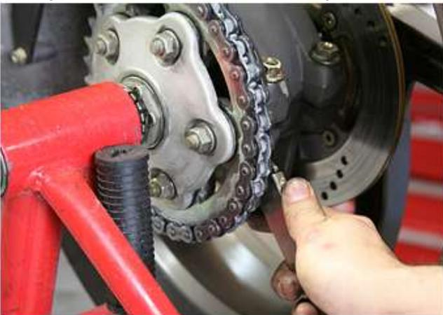
Chain tension is generally determined by the distance between the front and rear sprockets, and many bikes have index marks to help with alignment.
