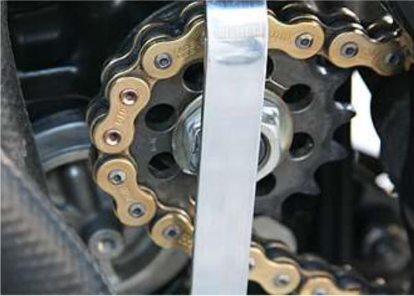
Front and rear sprocket teeth are good indicators of maladjusted chains; inspect the teeth to make sure they are meshing well with the chain. If the sides of the teeth are worn, chance is they haven't been seating well with the chain (which probably shows corresponding wear.) Wave-shaped teeth wear is another irregularity that might suggest that you need new sprockets.
