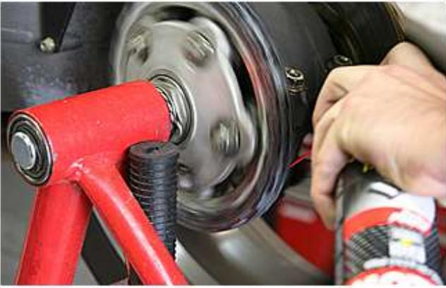
While rotating the wheel, evenly spray a layer of lubricant across the chain as it runs along the sprockets. Be sure to also spray at the bottom of the rear sprocket, where the lubricant can spread across the chain from the inside using centrifugal force, and penetrate the entirety of the chain. Wipe off excess lubricant with a rag.
