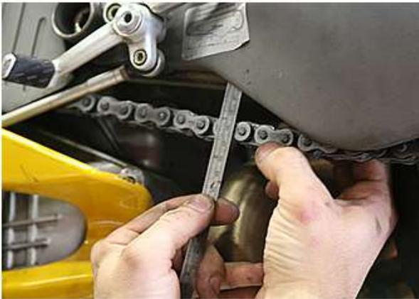
Using a tape measure (or visual estimation, if necessary), grasp the chain at a point halfway between the front and rear sprockets, and pull it up and down. The chain should be able to move roughly one inch up and one inch down. If your motorcycle is on a rear stand or centre stand, note that the swing arm will drop if the wheel is lifted from the ground, which will affect the rear geometry and the tension in the chain; compensate accordingly, if necessary.
