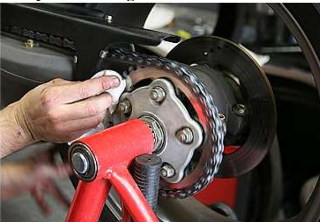
Next, you'll want to wipe off the excess grime using a rag or towel, which will create a clean surface that's friendlier to lubricants. Be sure to thoroughly reach all the sprocket teeth and chain links by rolling the rear wheel (or the entire bike, if it's not on a stand.)
